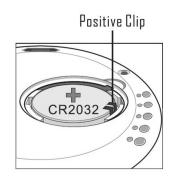
There are Positive Clip and Negative Clip in the battery compartment. Let the Positive Clip contact with battery "+", and Negative Clip contact with battery "-". Do not place both of the Positive Clip and Negative Clip under the battery to touch "-".
